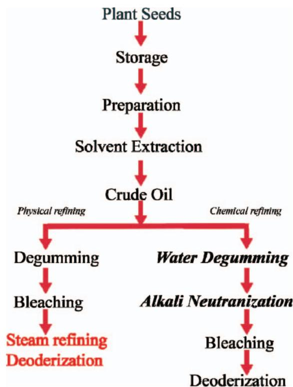
Figure 1 The schematic of oil refining process. (color figure available online.)
